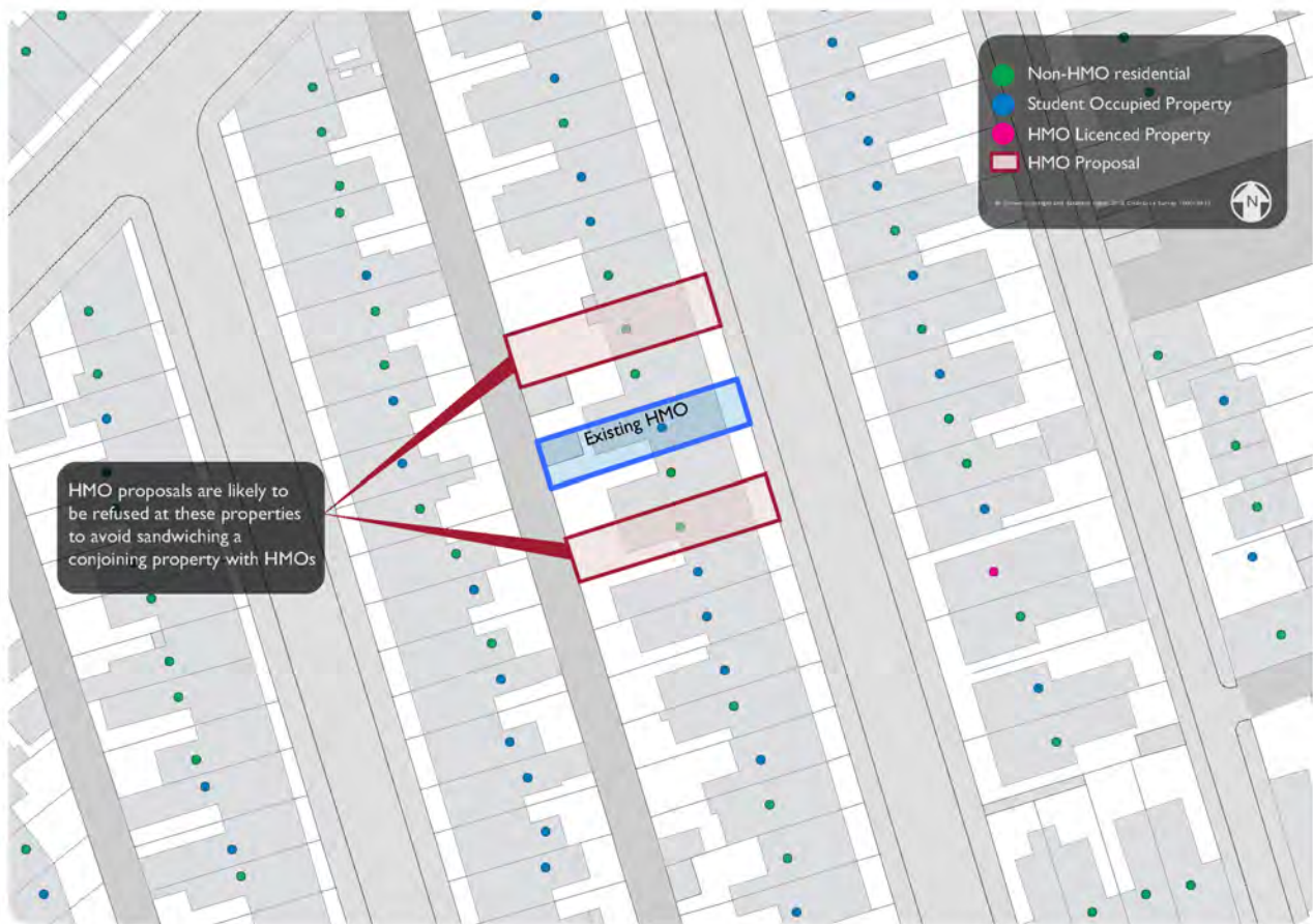
Figure 3 Illustration showing HMO 'sandwiching'
