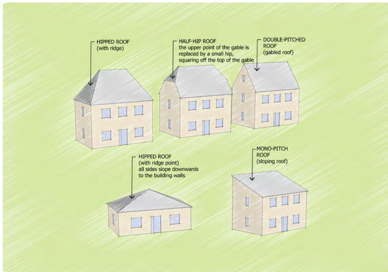
Figure 21 Technical terms for roof designs
