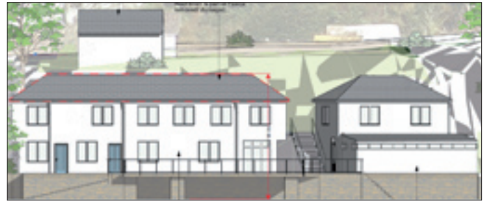
Existing building (above) height 9 metres from water level to roof apex (scale 1:100). Proposed building (below) height 14.3 metres from water level to roof apex (scale 1:200).
