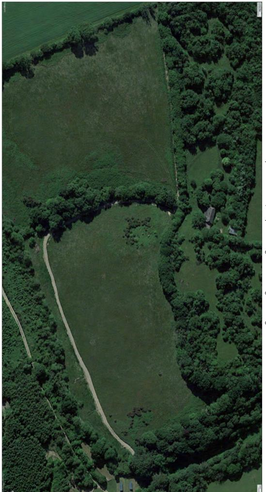
This Google Earth image, dated June 2022, clearly shows much of the track lies beneath the tree and hedgerow canopies. By being constructed so close to both, with no 2 metre protection zone, it is probable significant ecological damage will have occurred.
